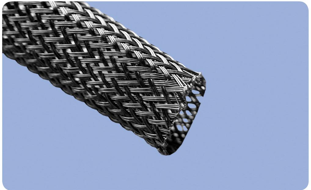
Bentley-Harris<sup>®</sup> Expando<sup>®</sup> products are tough, lightweight oversleeves used to protect cable assemblies, hoses and wire harnesses from chafing, cutting and abrading. The open-braid construction of Expando products enables each size to expand to fit several application shapes and sizes. This open-textile construction also makes them highly flexible and resistant to trapping water, heat and humidity.
