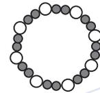
End view (enlarged diameter) of Expando DM showing nylon guard strands (larger) and polyester support strands (smaller, gray) in a typical configuration.
