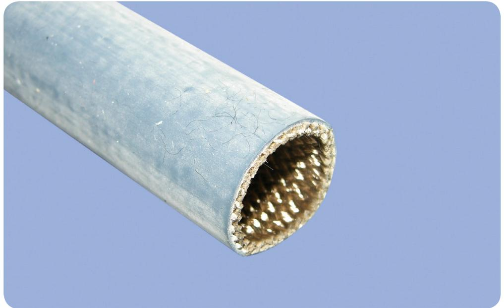
**Ben-Har™ 1151-FRB** is a rugged, flame-retardant, silicone rubber coated sleeving that provides excellent cut-through and abrasion protection for wiring systems in applications with temperatures ranging from -70°C to 200°C. Because the specially formulated silicone rubber is extrusion coated over the non-combustible fiberglass braid, it results in a reinforced sleeving that is superior to ordinary dip-coated sleeving and unreinforced rubber or plastic tubing.
